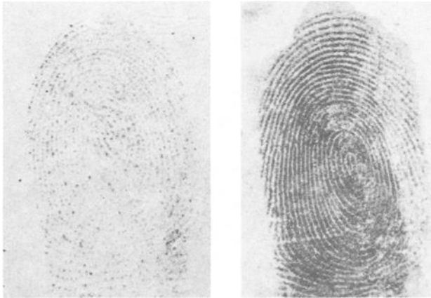
FIG. 5— Improved MCAR for the determination of latent fingerprints on paper (blood type B, secretor); (left) ninhydrin staining and (right) the MCAR pattern, obtained by improved method. Sensitization was done with anti-B, followed by MCAR with type B cells. The fingerprint pattern was definitely demonstrated by serological technique in comparison with ninhydrin method. No positive reaction (nonspecific adhesion of cells) was observed in cases in which the antigens and sensitizing agglutinins were incompatible.
